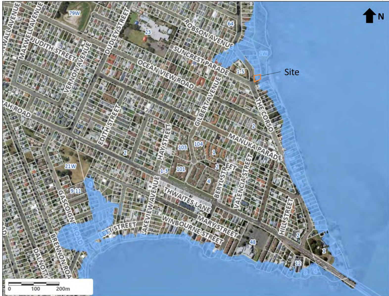
Figure 2: Flood extent of the 1% AEP lake flood (image based on Central Coast Council Online Mapping tool with flood level from Lawson and Treloar, 1994)
