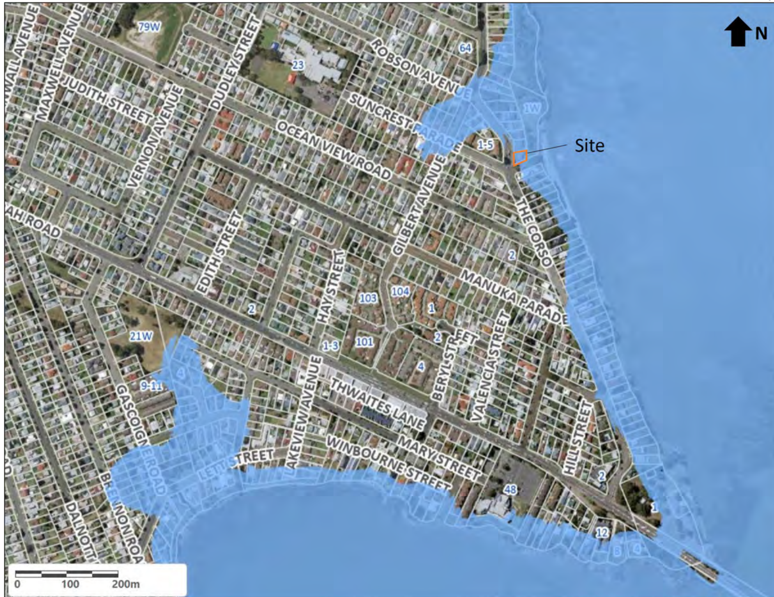
Figure 3: Flood extent of the lake flood PMF (image based on Central Coast Council Online Mapping tool with flood level from Lawson and Treloar, 1994)
